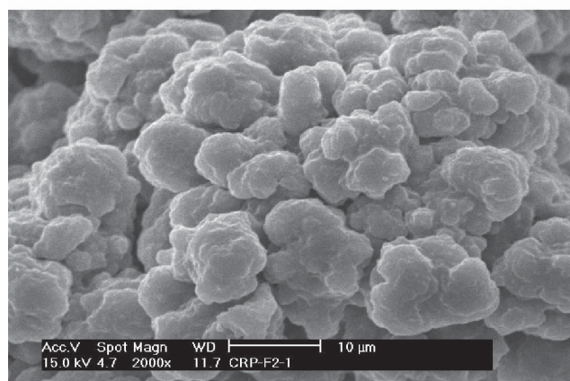
FIGURE 6. SEM photomicrographs of ASES-prepared microparticles bringing about coalescence and film formation at higher drug concentration in lipid carrier (8:2 (w/w)-PC:Chol): (A) 19% (w/w) Beta-val, (B) 19% (w/w) CRP.
